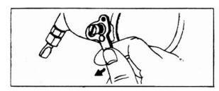
NOTE: On the model GP8000BS the choke is a ring tab located just under the engine air cleaner and must be fully extended during starting.
