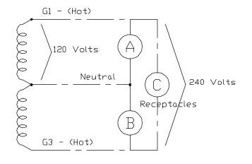
Check the appliance or tool nameplates for the current and voltage to insure compatibility. Remember that power taken from receptacle C reduces the power available at both A and B. Any remaining 120 volt loads should be equally divided between A and B. Failure to split the load will cause permanent damage to the stator. Although circuit breakers are provided, damage due to overloading constitutes abuse and will not be warranted.
