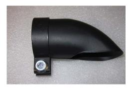
The exhaust deflector shown above was shipped loose with your unit. It is installed by sliding it over the exhaust pipe coming out of the muffler and tightening the locking ring. The exhaust can be direct in any direction.
