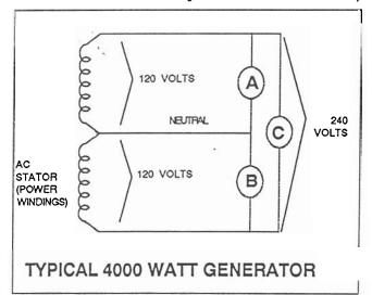
winding to allow the use of all the power available from the engine at either 120 Votts, 240 Volts or any combination of 120 or 240 Volts. You are not restricted to splitting up your large 120 volt loads or choosing to power them OR a 240 Volt load. There are no switches or connectors to change. Simply plug in and use the power without being concerned about overloading the generator.
